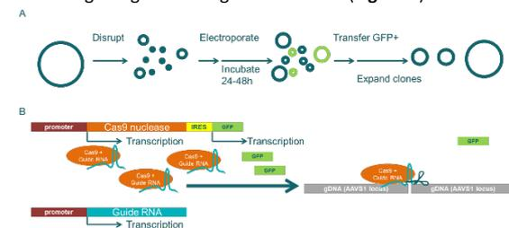
Figure 1. Overview of the experimental procedure. A: Schematic overview of the handling of Organoids to obtain CRISPR/Cas9 modified clones. B: Graphical representation of transient expression construct used to achieve targeted modification of the AAVS1 Locus.
